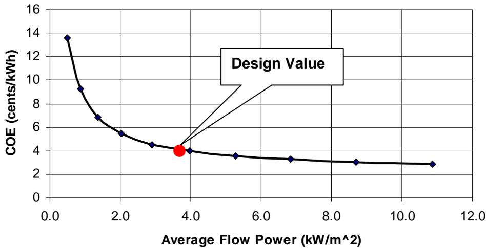
Figure 53 – Sensitivity of COE to average flow power in kW/m<sup>2</sup>
