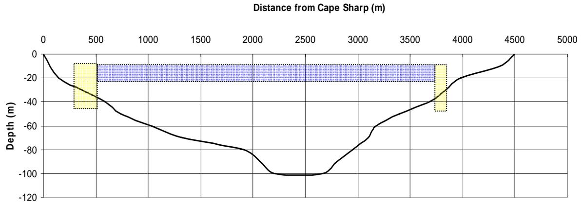
Figure 46 - Channel Cross section at Cape Sharp
