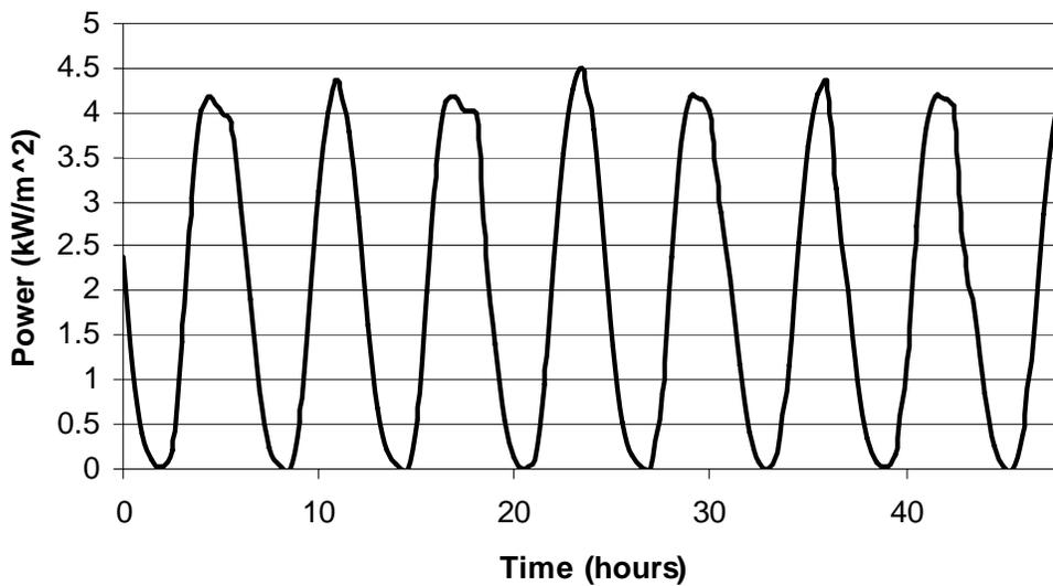
Figure 6 - Depth averaged power density over 48-hour period at Cape Blomidon Transect
