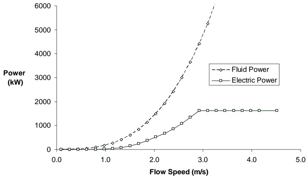
Figure 24 – Comparison of water current speed and electrical power output
