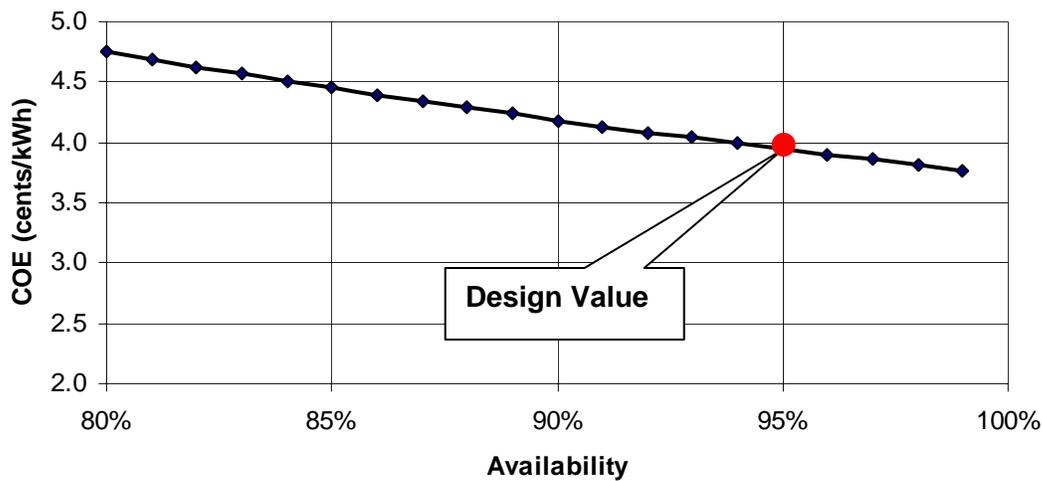
Figure 52 – Sensitivity of COE to array availability
