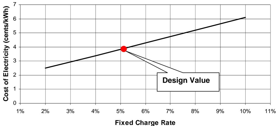
Figure 56 – Sensitivity of COE to Fixed Charge Rate
