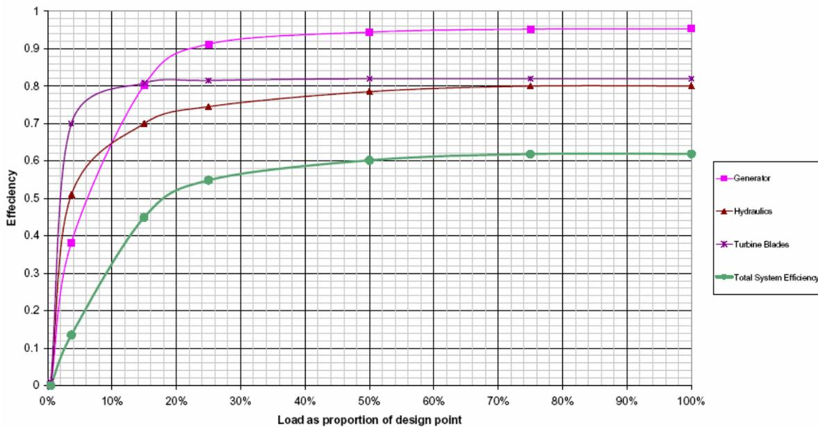
Figure 23 - Efficiency curves of Power Conversion System
