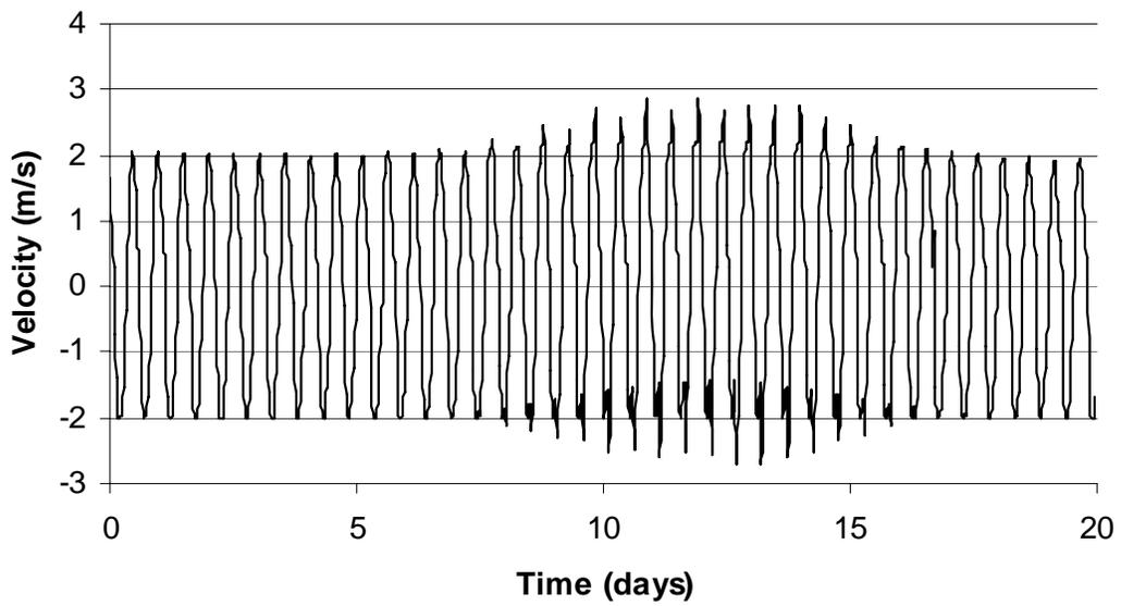
Figure 8 - Depth averaged velocity at Cape Blomidon over a full lunar cycle
