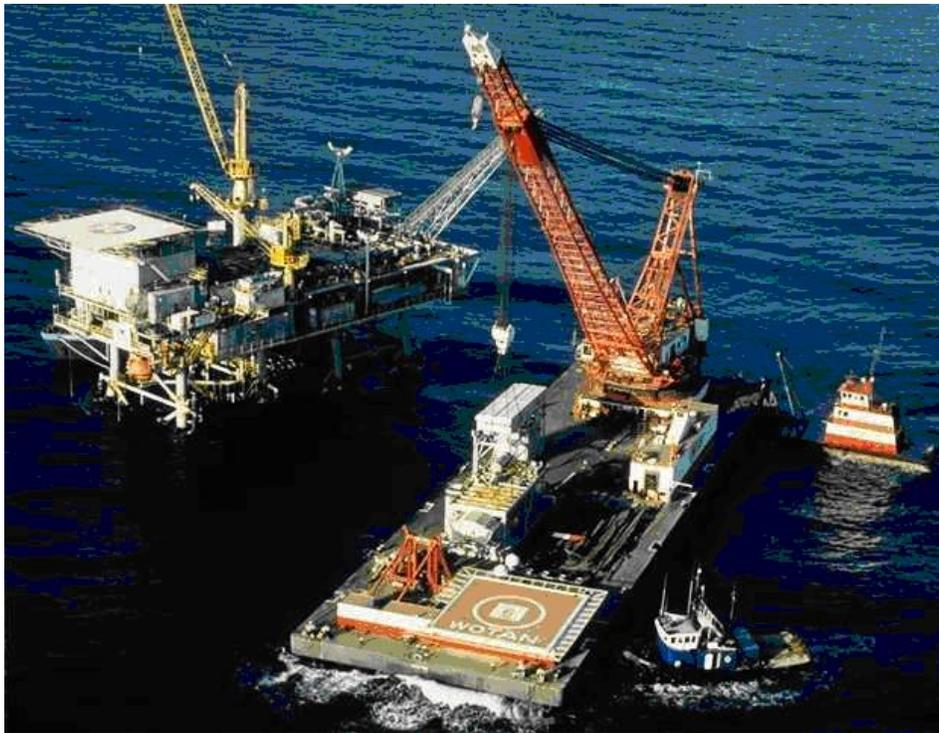
Figure 28 - Manson Construction 600 ton Derrick Barge WOTAN operating offshore
