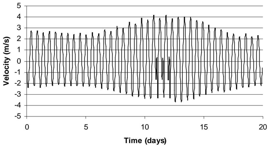
Figure 14 - Depth average velocity over full lunar cycle
