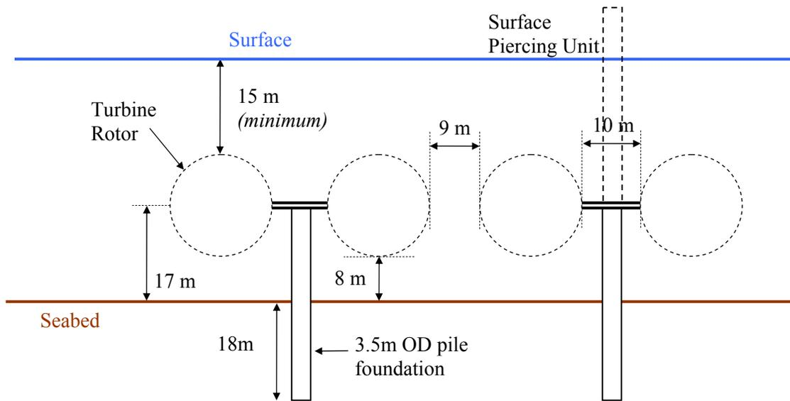
Figure 47 – MCT SeaGen Turbine Spacing Assumptions
