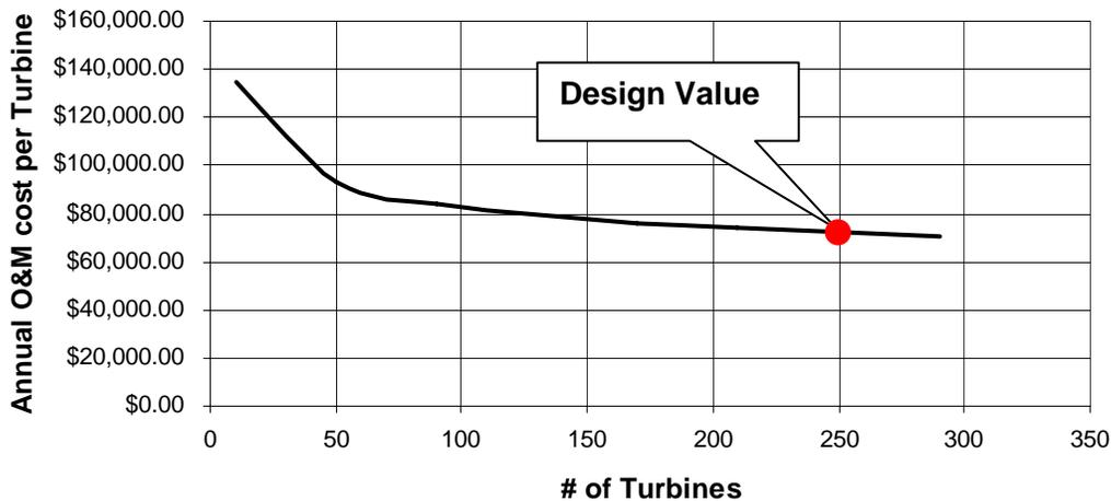
Figure 51 – Sensitivity of annual O&M cost to number of installed turbines
