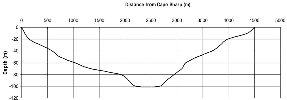
Figure 17 - Cape Sharp channel cross section
