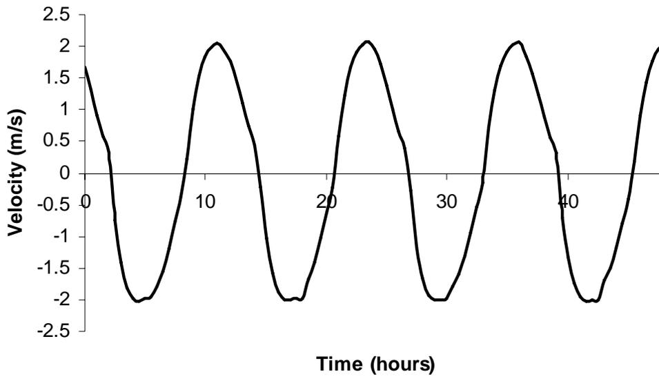
Figure 5 - Depth average velocity profile at the Cape Blomidon Transect
