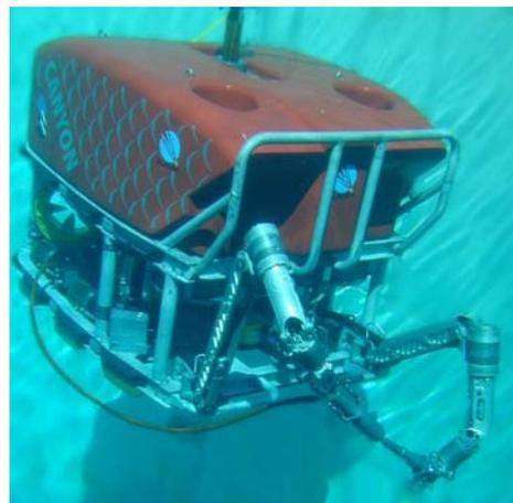
Figure 29 – Remotely Operated Vehicle (ROV) – (courtesy of Schilling Robotics - [www.ssaalliance.com](http://www.ssaalliance.com))
