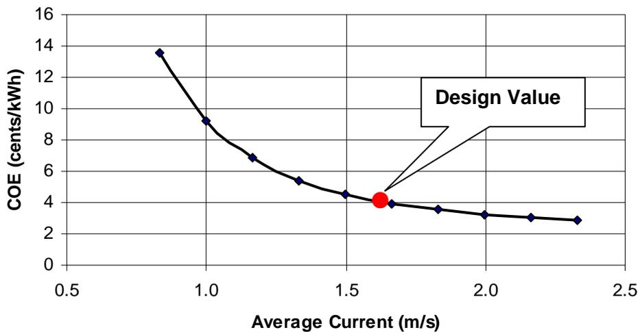
Figure 54 – Sensitivity of COE to average current speed (m/s)
