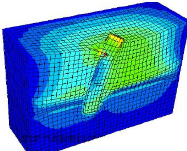
Figure 37 - Simulation of pile-soil interaction subject to lateral load (Source: Danish Geotechnical Institute)
