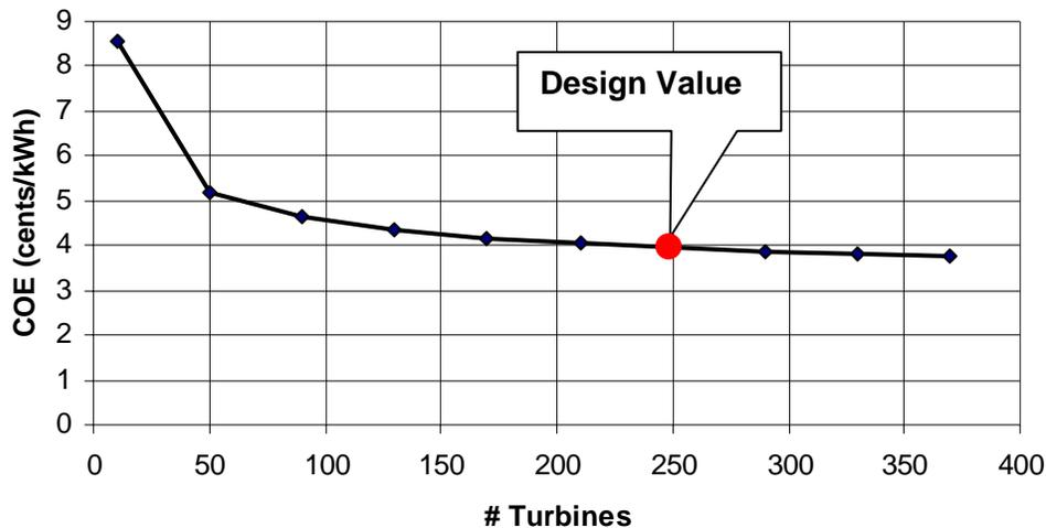
Figure 49 – Sensitivity of COE to number of turbines installed
