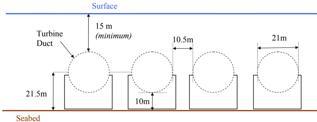
Figure 48 - Lunar RTT 2000 Spacing Assumptions
