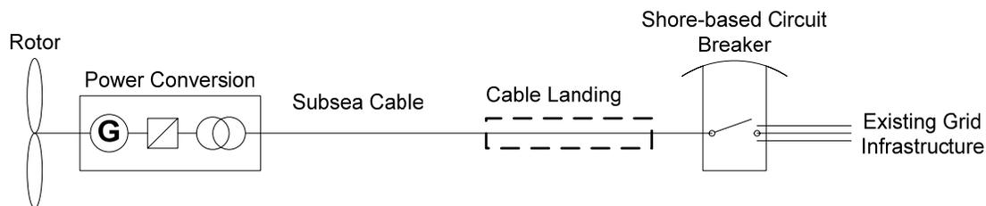
Figure 43 - Conceptual Electrical Design for a single TISEC Unit
