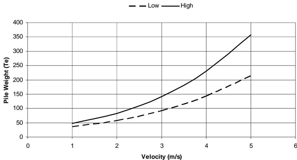
Figure 38 - Pile Weight as a function of design velocity for different sediment types
