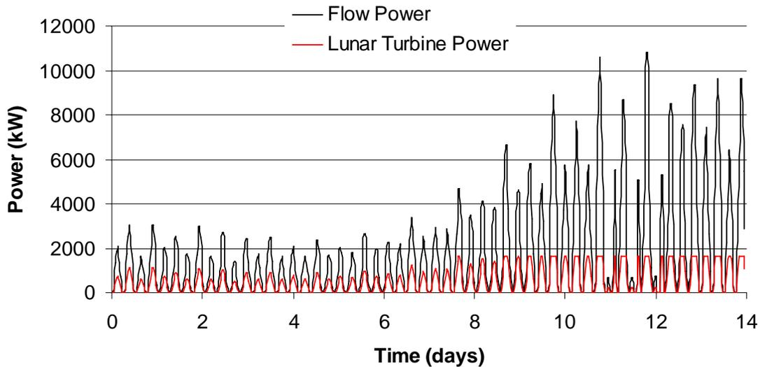
Figure 26 - Flow power vs. electrical power output at the site
