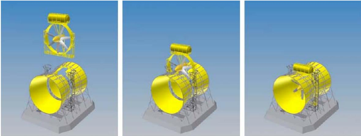
Figure 22 - Insertion and removal of cassette
