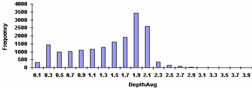
Figure 4 - Depth averaged velocity distribution at the Cape Blomidon demonstration plant site. Velocity shown is in m/s.
