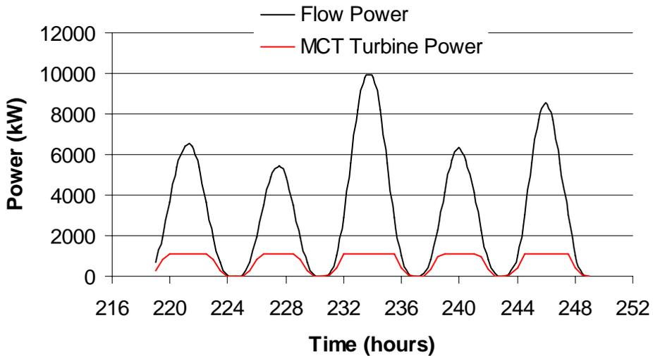
Figure 33 – Variation of flow power and electrical power output at the site
