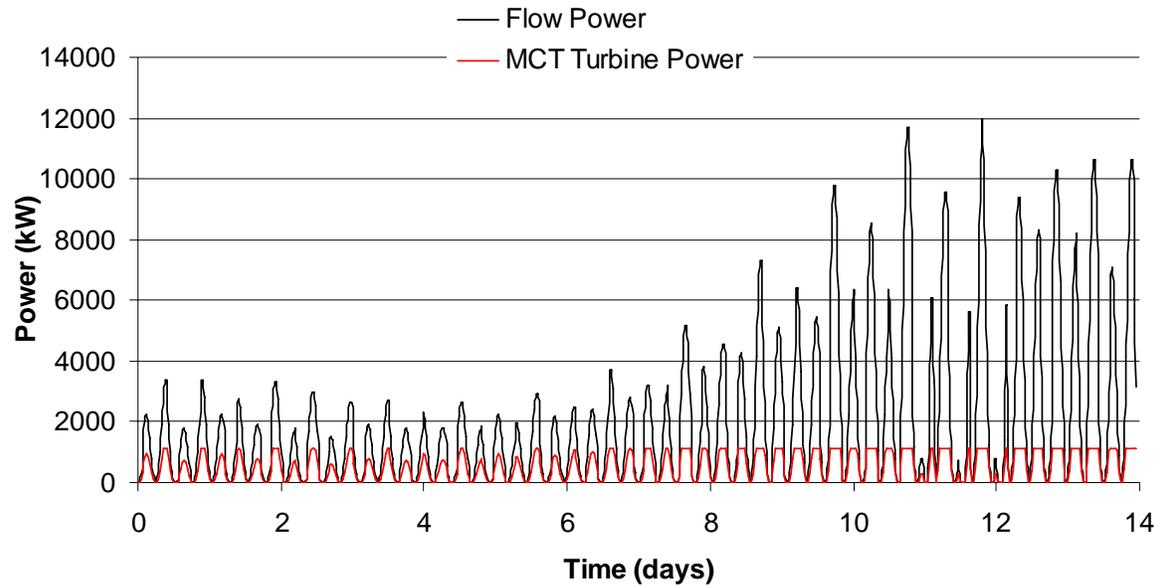
Figure 34 - Device power vs. flow power in cross sectional area of device
